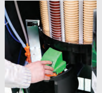
Daily maintenance items are clearly marked in green.
